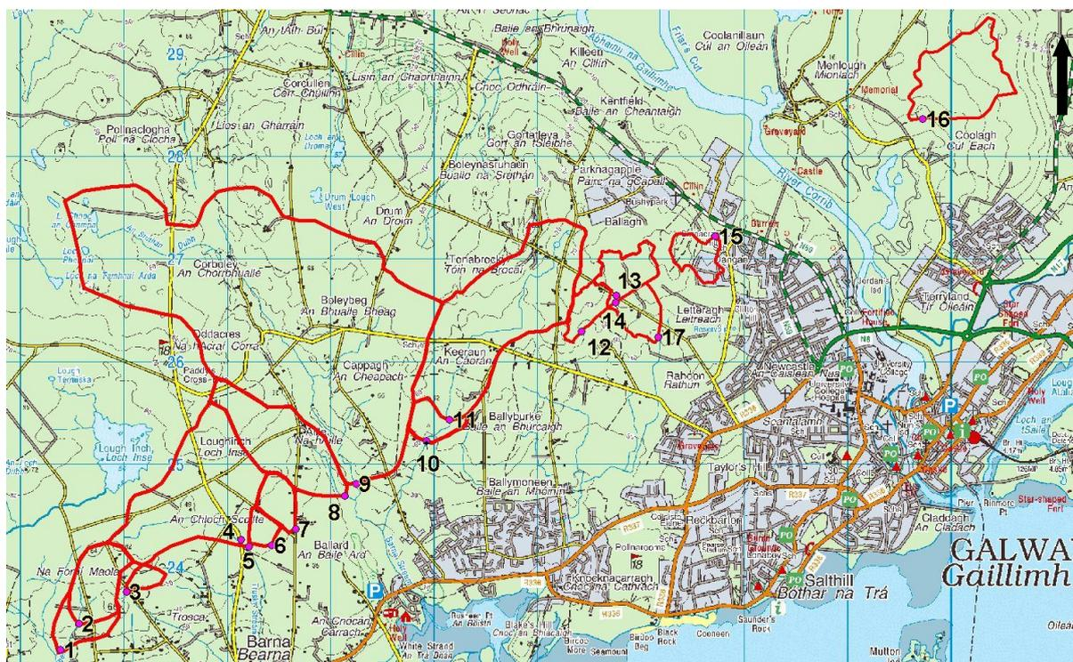
Figure 5 Contributing Catchment Area of Culverts (red polygons)
